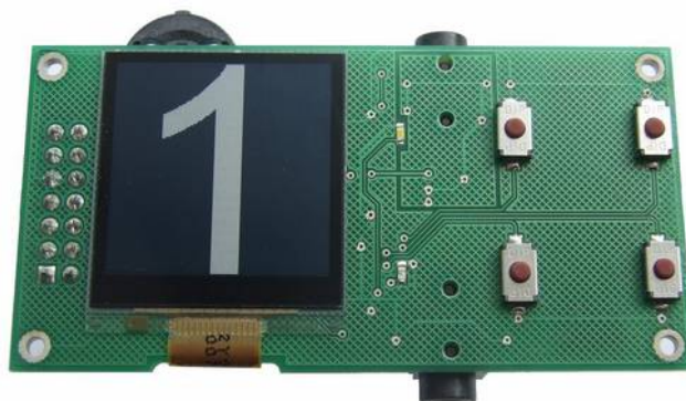
Figure 8. FFTD1A showing a sequence of images direct from FLASH program memory
